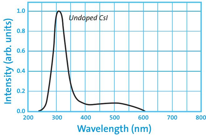
Figure 1. Scintillation emission spectrum of CsI(pure)
